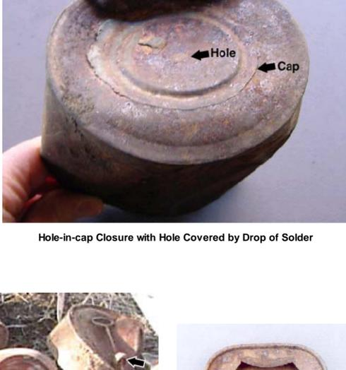
Hole-in-cap Closure with Hole Covered by Drop of Solder
