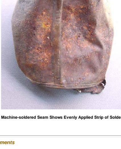
Machine-soldered Seam Shows Evenly Applied Strip of Solder
